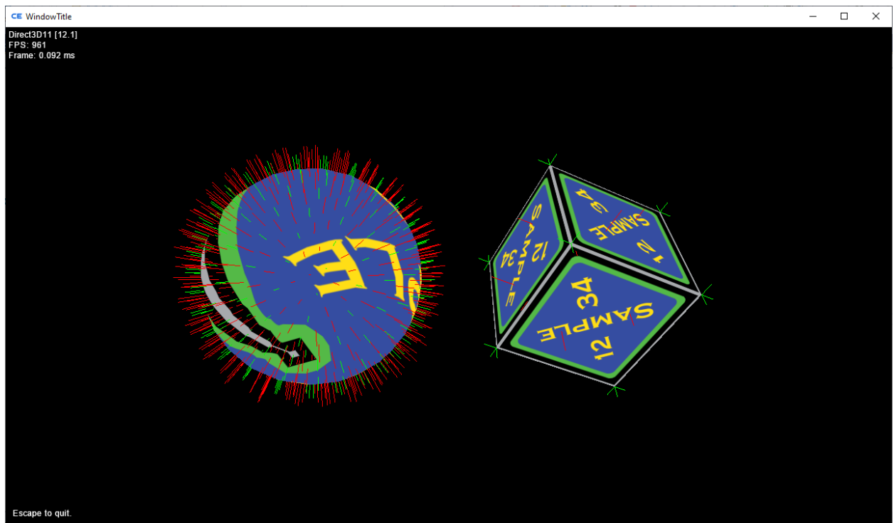
Figure 30 Example of a geometry shader rendering the normals of the points and face of triangles.
